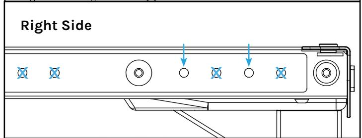
C. Using the 5mm Allen Wrench, insert two of the M8 x 10 Button Head Screws in the threaded holes shown in the image leaving a gap of about 1/4" (5mm) between the frame and underside of the screw head.
