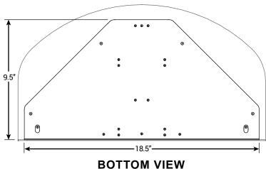
The bottom plate is smaller than the top, and is the surface to which the Keyboard Tray is attached
