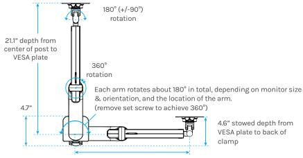
18.3" Side Extension - from center of base to center of VESA plate
