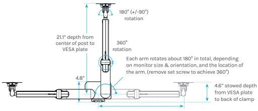
20" Side Extension - from center of base to center of VESA plate
