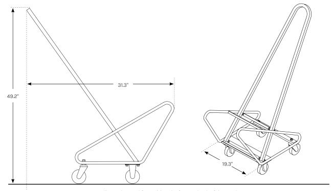
Dolly can be used from either the front or back of the stack.
